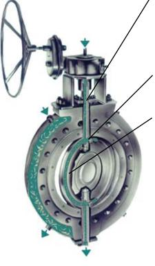
The shaft of any valve is especially vulnerable to media build-up. Even a small amount of flow material solidifying on the bearing surface can cause binding and wear. With the unique Tufline HPBV-STJ design, steam flows directly through the stem, fully heating the bearing area. Optional purge and sealed-bearing configurations are also available.
