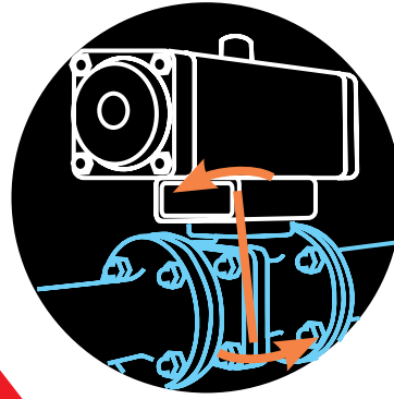
Actuation loads and misalignment
