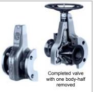
The radius clamps are connected to the yoke and to the compressor by means of links and link pins. These components, working together, provide a scissor-jack action which pushes the tube element inward during the opening cycle and pulls it outward during closing. Four lift forks imbedded top and bottom in the tube element on each side of the clamp act as powerful fingers which work with the links and link pins to pull the sealing surfaces apart even under full vacuum conditions.
