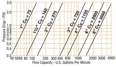
C<sup>v</sup> is a coefficient which relates the rate of fluid flow through a valve to the pressure drop across the valve. Valves with higher values of C<sup>v</sup> will provide higher rates of flow for a given pressure drop. C<sup>v</sup> values for PTFE Clamp Valves are dependent upon inlet pressure. C<sup>v</sup> values shown above were determined with inlet pressure of 65 psi or higher.
