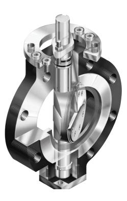
angle that is inclined from the center line of the valve bore to minimize rubbing of the seat/seal contact surfaces during operation, and to preserve sealing integrity over the cycle life of the valve. This unique design can accommodate the temperature extremes present in gas applications, from cryogenic to extremely high temperatures.
