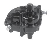
Matryx<sup>\*</sup> Vane Actuators. Matryx Vane Actuators provide the most reliable and efficient remote control of any type of rotary operation. They are used for ball, plug, and butterfly valves as well as other mechanisms such as dampers, switches, and safety devices. They are available up to 30,000 in-lbs of torgue.
