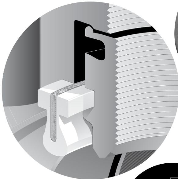
The patented seat is axially pliant. Unlike other seats, there is no radial stretch. When the valve opens, the seat flexes axially, returning to its original compact shape. It does not "relax" into the flow path.
