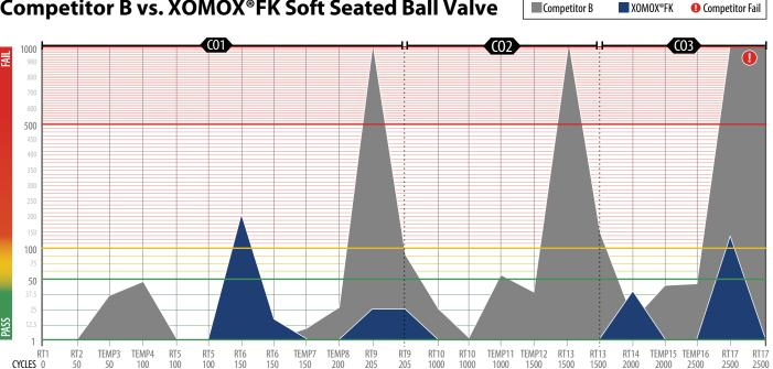
Note: Adjustments made at any peak over 50 ppm. Per ISO 15848-1, one adjustment is allowed per each endurance class.
