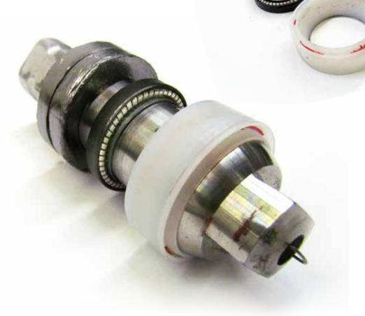
This valve incorporates three independent stem seals. 1st seal is the patented pressure-assisted SX chemically modified PTFE stem seal, 2nd seal is a spring energized (live loading) lip seal Carbon filled PTFE, 3rd seal is graphite packing. No visible extrusion of any of the three seals.
