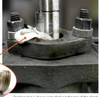
Packing ring is shown extruded out the top of the gland follower and around Stem O.D. causing stem leakage.
