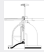
Non-rising handwheel with indicator DN200 - DN350 8" - 14"
