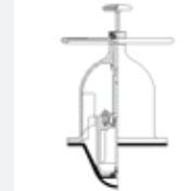
Non-rising handwheel with indicator DN200 - DN300 8" - 12"
