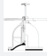
Non-rising handwheel with indicator DN200 - DN350 8" - 14"
