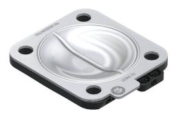
Saunders<sup>®</sup> SR and PR diaphragms feature the Saunders<sup>®</sup> bayonet type compressor attachment which allows the diaphragm to float freely relative to compressor to avoid point loading of the TFM at the stud. The bayonet fit also facilitates easy error free engagement of diaphragm and compressor.
