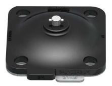
The Saunders® SR diaphragm features the Saunders® bayonet type compressor attachment which allows the diaphragm to float freely relative to compressor to avoid point loading of the TFM at the stud. The bayonet fit also facilitates easy error free engagement of diaphragm and compressor.
