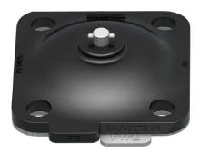
The Saunders® PR diaphragm features the Saunders® bayonet type compressor attachment which allows the diaphragm to float freely relative to compressor to avoid point loading of the PTFE at the stud. The bayonet fit also facilitates easy error free engagement of diaphragm and compressor.
