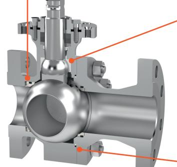
Alternatively, for higher temperature applications, Krombach offers a graphite packing arrangement with metallic diffusion barrier rings to ensure the highest levels of fugitive emissions containment without sacrificing LOW TORQUE OPERATION and Fire Safe protection.
