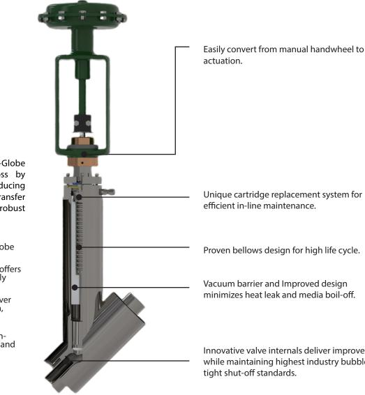
Crane CRYOFLO® Bellows Seal Y-Globe Valves minimizes Hydrogen loss by improving heat transfer rates, reducing pipeline latency in liquid transfer applications and leveraging a robust zero-leak design.
