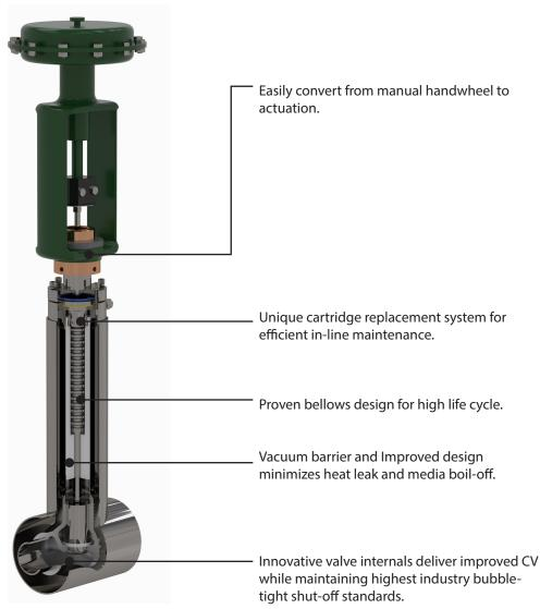
Crane CRYOFLO<sup>®</sup> Bellows Seal T-Globe Valves minimizes Hydrogen loss by improving heat transfer rates, reducing pipeline latency in liquid transfer applications and leveraging a robust zero-leak design.
