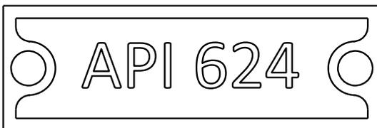
Valves with a prefix "L" in figure number will have an API 624 tag riveted to the valve. This tag designates the valve meeting API 624 for low fugitive emissions.
