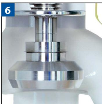
**6** Exchangeable disc with conical shape; **sealing surface hard-faced** with Stellite® 6; **body seat hard-faced** with Stellite® 21
