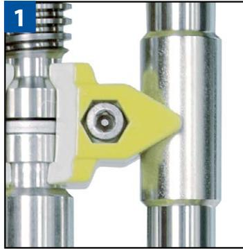
Safety **gland packing** made of graphite; gland follower with double wiper or O-ring seal made of FKM
