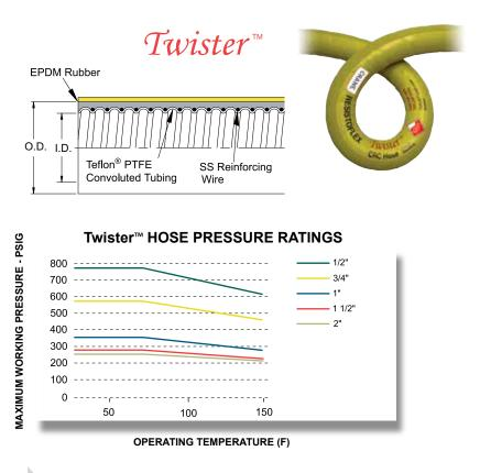
NOTE: For assemblies, pressure ratings of fittings may be less than for the hose.
