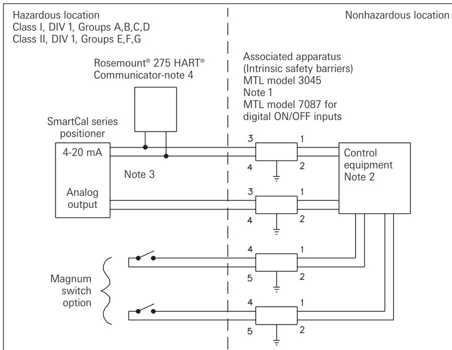
1. Associated apparatus manufacturer's installation drawing must be followed when installing this equipment.
