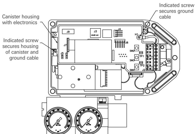
**Appendix C - Setting the transmitter output fail current**
