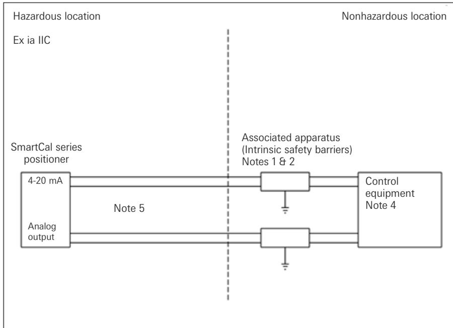
Entity parameters for each field wiring terminal pair of SmartCal:
