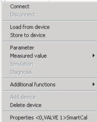
Before starting configuration of the SmartCal, you must download the current configuration. Select <connect> and <load from device>. All parameters are now downloaded from the SmartCal and are available for editing.
