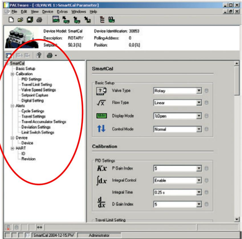
With the Basic Setup menu you can configure the settings for Valve Type, Flow Type, Display Mode and Control Mode.
