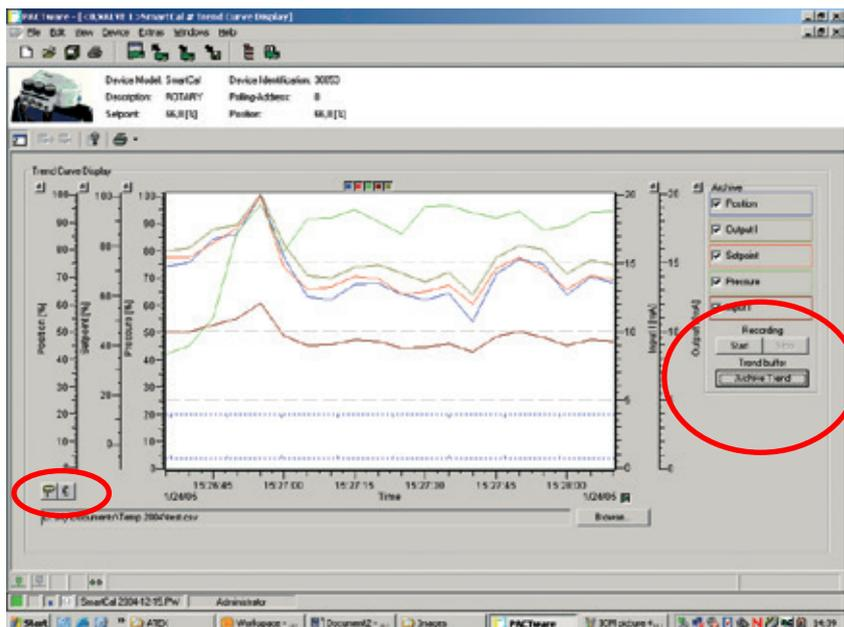
The left-hand and right-hand mouse buttons are used to set the y-axis. The icons on the lower left are used to simply capture the values in the graph.
