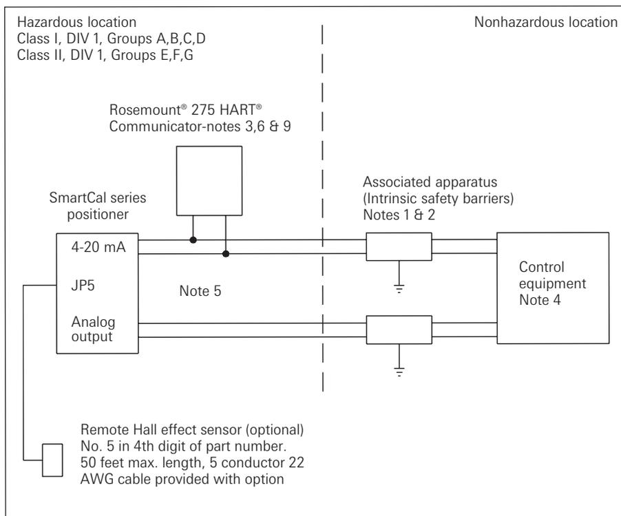
Entity parameters for each field wiring terminal pair of SmartCal:
