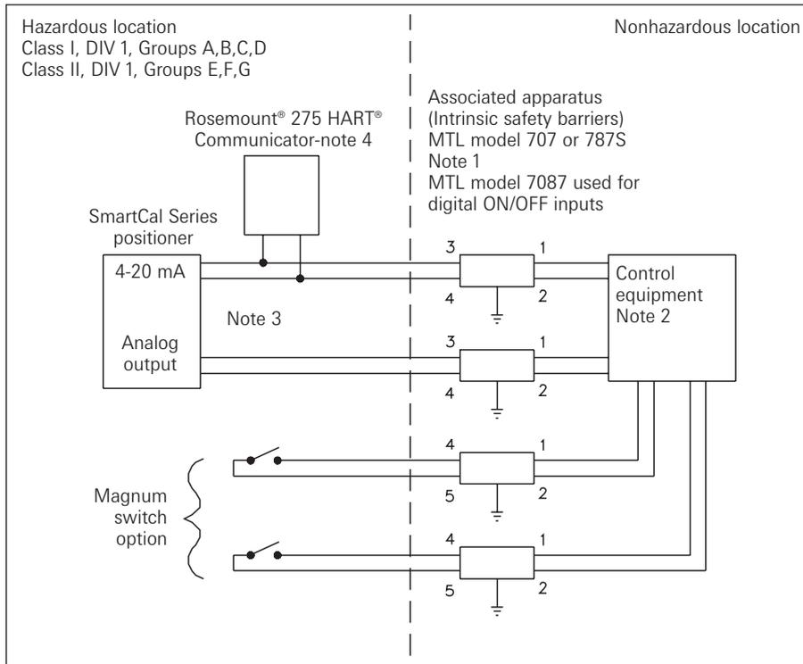
1. Associated apparatus manufacturer's installation drawing must be followed when installing this equipment.
