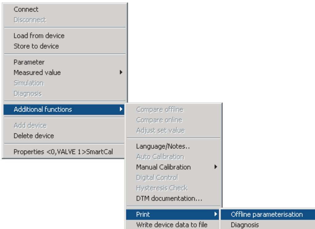
If you have completed the full configuration of the SmartCal, recommends making a copy of all parameter values. The parameters are saved in the FDT application. However, a hardcopy can be obtained by the 'Print Offline Parameterization' function. This offers a complete overview of all available parameter values. The print-out can also be saved in Microsoft Word. Select 'Print' and select all values with by <CTRL> + A and paste the selection into a Word file.
