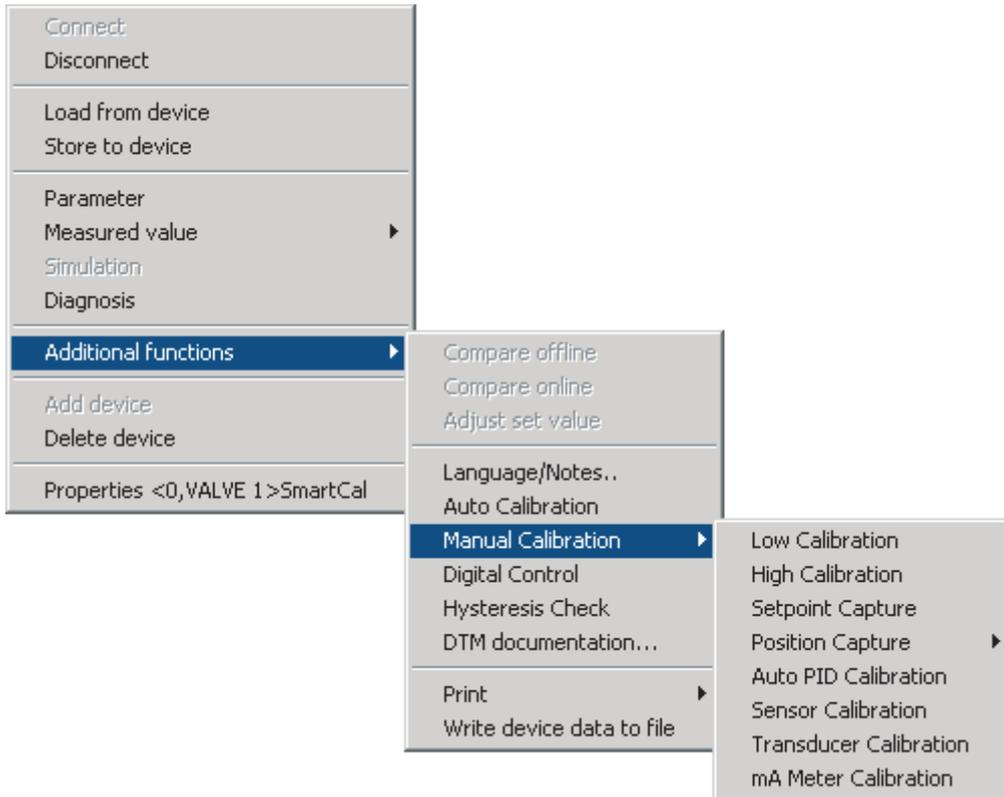
The 'Additional functions' offer the possibility to execute a complete auto calibration or any manual calibration. Please note that calibration cannot take place during normal process conditions. If you use a HART® network, be sure to select the correct device.
