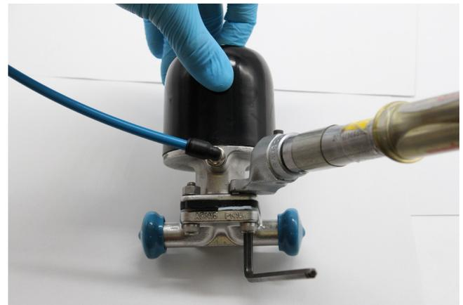
10. Gradually tighten the fasteners as per figure 1 to approximately 3/4 of full torque. (See torque specification table). This ensures that the diaphragm seats correctly before further tightening
