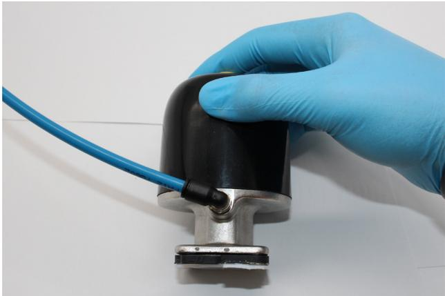
Remove the fasteners and the valve actuator
