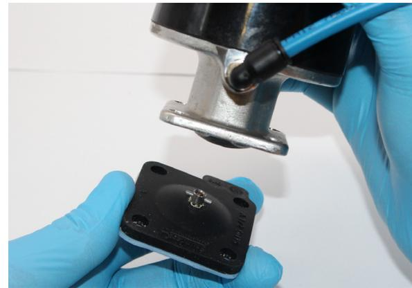
Remove Diaphragm From Actuator
