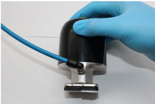
Engage diaphragm bayonet into the compressor slot by applying pressure to the centre of the diaphragm. Ensure correct engagement and continue to apply pressure to the centre of the diaphragm and turn through 90°
