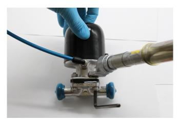
**10.** Gradually tighten the fasteners as per figure 1 to approximately 3/4 of full torque. (See torque specification table). This ensures that the diaphragm seats correctly before further tightening
