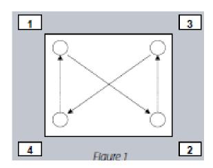
Attach the actuator to valve body; Insert the retaining fasteners. Hand tighten fasteners in the order shown in Figure 1.
