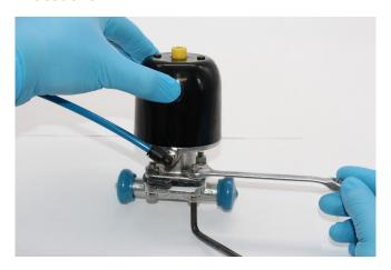
Start to loosen the fastenings Important: Ensure the excess pressure has vented prior to fastening removal
