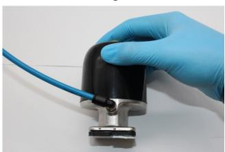
Remove the fasteners and the valve actuator
