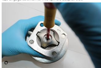
**16.** Unwind the spindle adaptor releasing the compressor
