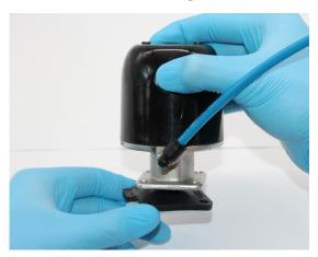
Ensure actuator is in the closed position: Release air pressure on NC Actuators
