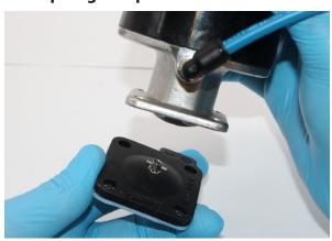
Remove Diaphragm From Actuator
