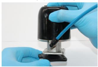
Engage diaphragm threaded stud into the compressor by applying pressure to the centre of the diaphragm. Ensure correct engagement and continue to rotate clockwise until resistance felt. Rotate diaphragm anti-clockwise until diaphragm bonnet hole alignment is achieved
