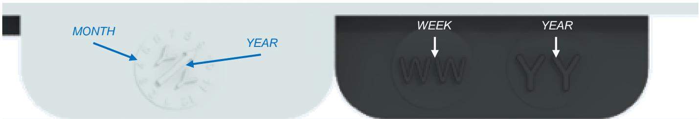
*Diaphragm tab to always face towards you on both Rubber (Elastomer) and PTFE style diaphragms*
